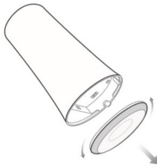
Step 2: Insert Ethernet cable (PoE) for power & isolated ground cable for safety. Reinstall bottom cap
