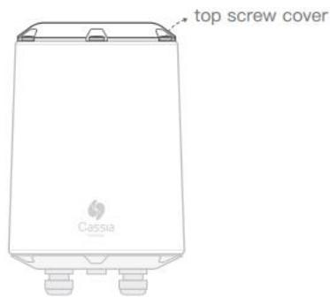
Step 2: Use cross screwdriver to open the top cap
