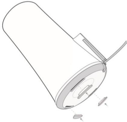
If the user wants to ground the gateway, there are many different types of cable diameters and cable hardness levels. When a grounding cable and Ethernet cable are used together, the resulting thickness might prevent silicone plug from sealing 100%.
